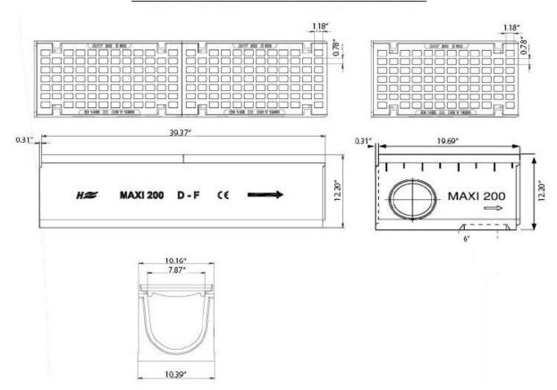
MAXI 7.87" [200] wide throat **Ductile Iron Grate is rated class E** per the DIN EN1433 top load classifications. Ductile Iron conforms to ASTM specification A536-84, Grade 80-55-06. Supplied in 39.37" [1000] or 19.69" [500] nominal lengths with 1.18/0.78 [30/20] wide slots. Grate has an open area of 49.13 sq. in per ft. [104,006 sq.mm per meter].
